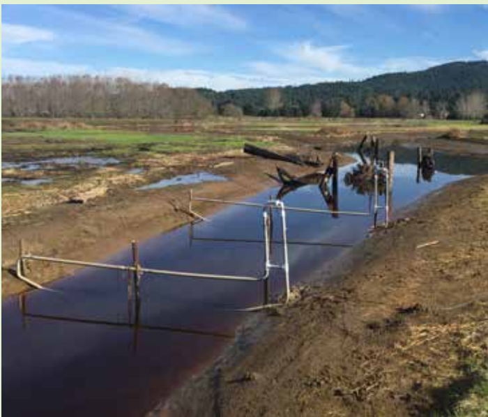
Wood Creek restoration antennae detecting tagged fish using new habitat.
